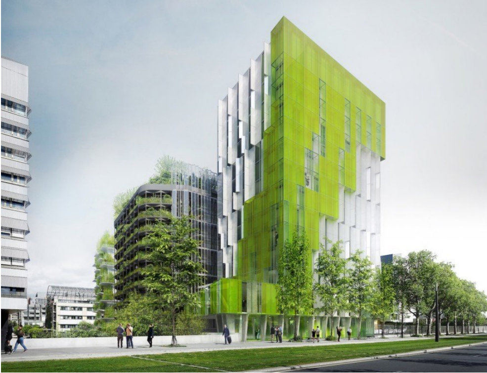
Figure 8. Solar powered algae bio-facade “Vivo”, designed by XTU Architects.
